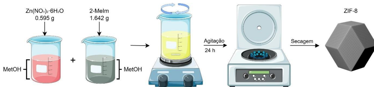
Figure 15 – Schematic illustration of the synthesis procedure for ZIF-8
