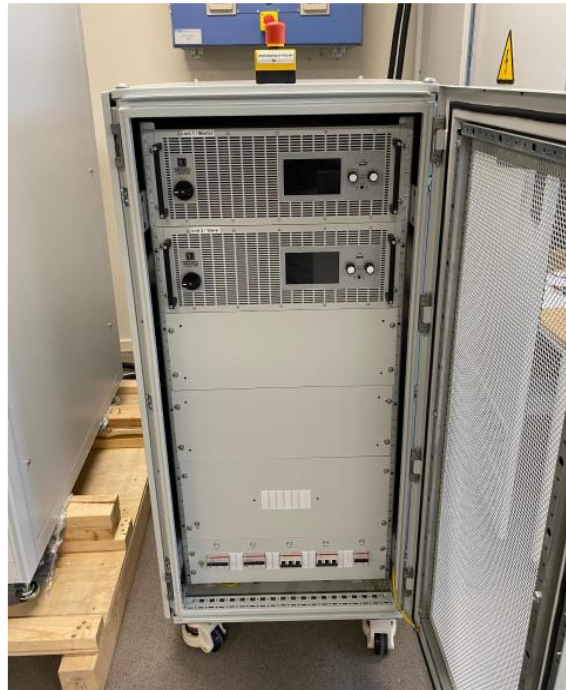
Figure B-5 – DC voltage source.
