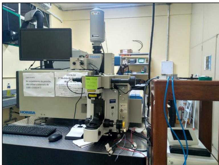
**Figura 24** – Espectrômetro Raman Horiba Jobin-Yvon T64000
